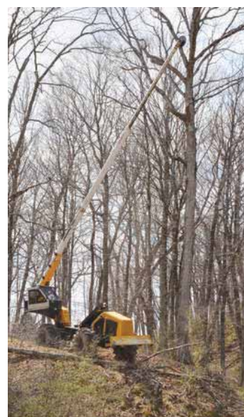
EnerStar's ROW plan included a visit from the "giraffe," which is actually a Jaraff — a mechanical tree trimmer. This machine features a long, extendable boom with a circular cutting blade that can rotate 180 degrees for precise cuts in any direction. It can reach heights of up to 75 feet and trim up to 1,000 feet per day.
