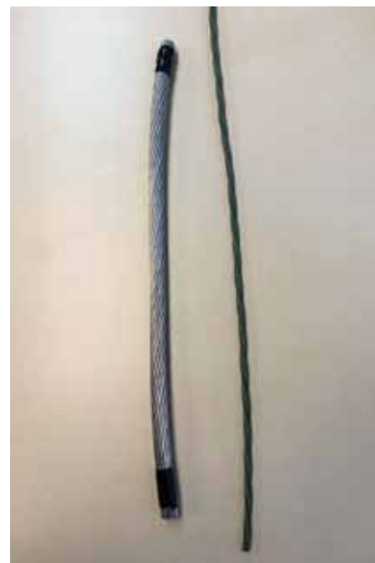
The 336 ACSR wire (left) will be replacing the 4A Copperweld (right) in some areas as part of CCEC's construction work plan.
