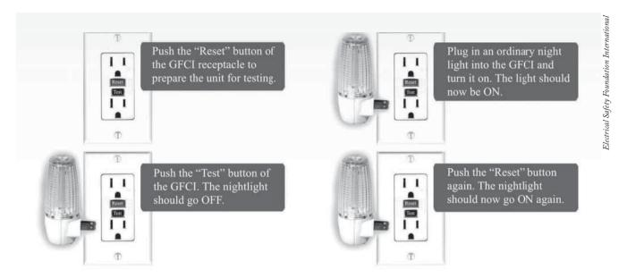
Since the 1970s, ground fault circuit interrupters (GFCIs) have saved thousands of lives and have helped cut the number of home electrocutions in half.
