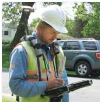
This field technician enters data on a tablet computer while the GPS device on his back records the location.
