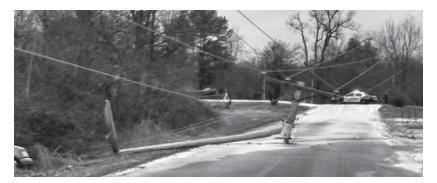
What would you do if you hit a utility pole and the lines and pole came down on or around your vehicle? Stay inside until help arrives! (Unless the vehicle is on fire). If you have to get out, jump away from the vehicle with both feet together, as far away from the vehicle as possible (like a bunny hop). Getting out of the vehicle, with few exceptions, is the wrong thing to do until the line has been de-energized.
