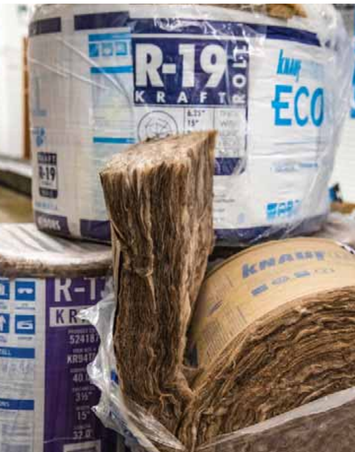
There are different types of insulation, including fiberglass batts, blown fiberglass, cellulose and foam. Each has its own R-value, which is listed on the packaging. Photo courtesy of Mark Gilliland.
