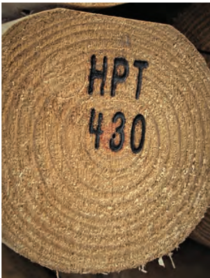
Manufacturer's code, class and length are also printed on the ends of each pole for easy identification.
