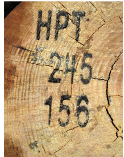
Manufacturer's code, class and length are also printed on the ends of each pole for easy identification.
