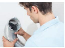
line—it should not have a lot of slack. with twists and curves. A shorter, unobstructed vent hose increases the efficiency of your dryer, dries clothing faster and reduces lint buildup, which can create potential fire hazards.
