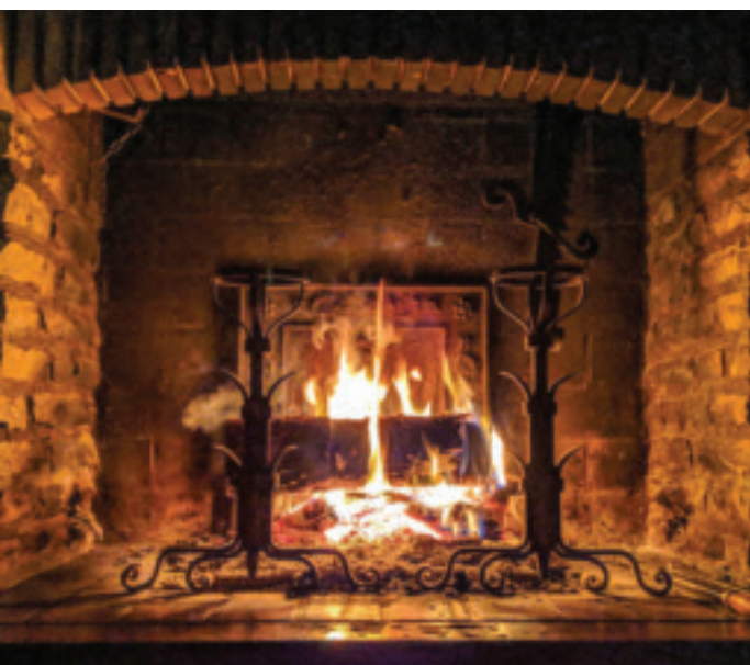
Burning wood produces radiant heat, which feels great if you're near the fire, but it can also send large amounts of room air up the chimney.
