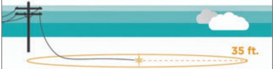
Downed power lines can energize the ground up to **35 ft.** away - so keep your distance.
