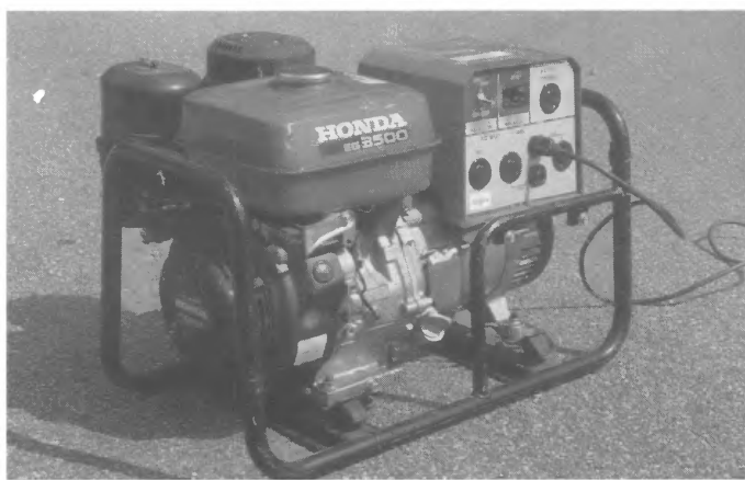
Plugging appliance cords directly into a portable generator is an accepted practice.
