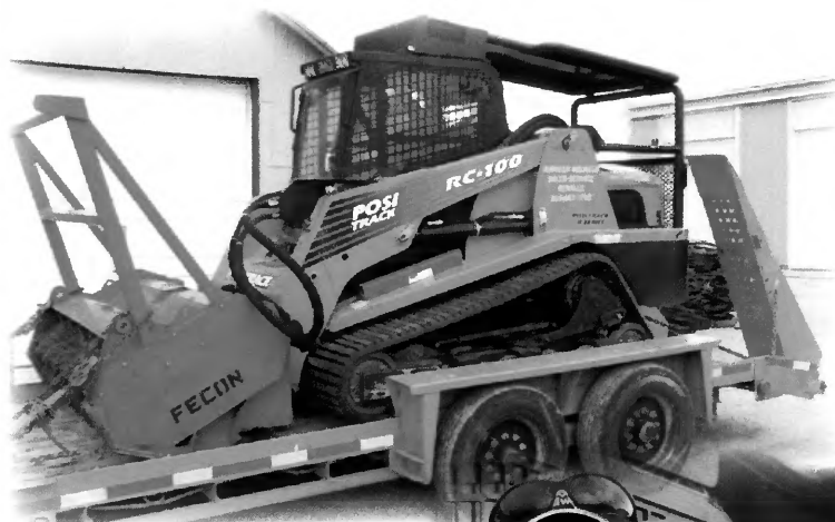
This machine can cut down and chip an 8-inch by 30-foot tree in a matter of minutes.
