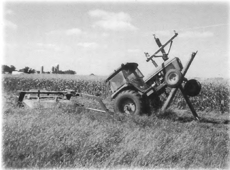
Don't make this mistake. Stay clear of guy wires. Accidentally hitting guy wires weakens the support for utility poles. Know the height of all equipment and stay at least 10 feet away from overhead lines. Never attempt to raise or move a downed power line.
