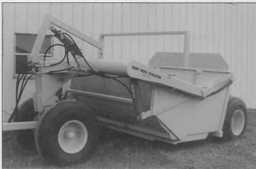
▲ Weighing in at approximately 6500 pounds, the Dirt Hog is mounted on C-130 air transport plane tires.
