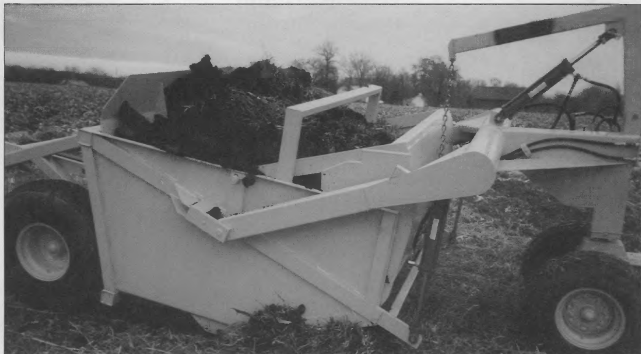
▲ The Dirt Hog in action: The bin has a capacity to hold a full 8 yards of dirt or dirt-sod combination.
