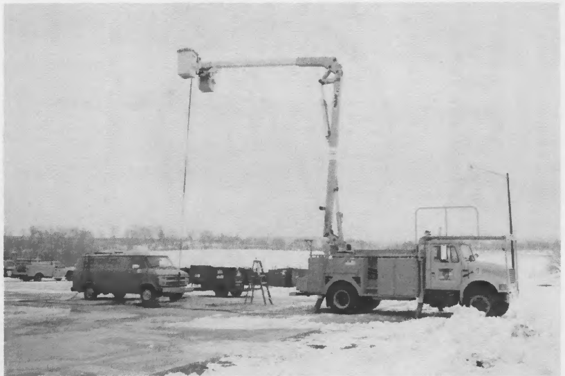
The firm of Quad-City Testing Lab tests one of Jo-Carroll's aerial trucks for safety compliance. This firm measures the dielectric strength and the mechanical strength of all of Jo-Carroll's equipment each year, to ensure that our linemen are able to work safely.
