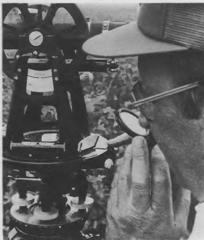
Peterson using a magnifying glass to read the angle on a line adjustment.
