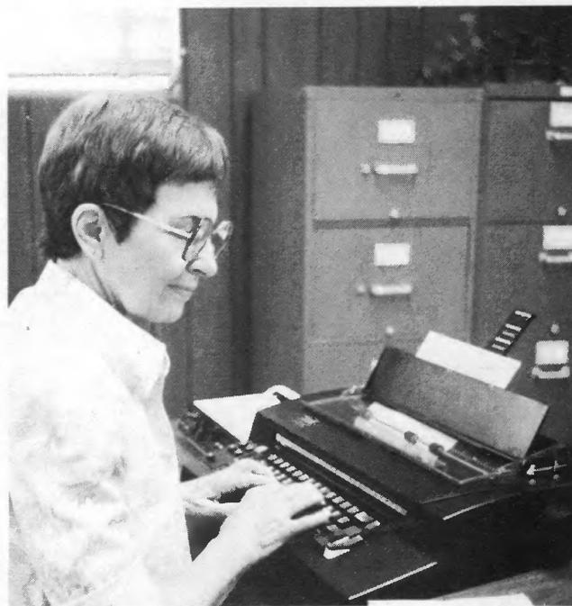
Fern Newton, Secretary to the Manager, at her new electronic typewriter which has a memory and in itself is a small computer. The typewriter memory stores typewritten material that can be used to type identical material automatically. The storage capability eliminates much retyping when copy is revised. Errors are easily corrected and columns of numbers automatically aligned.
