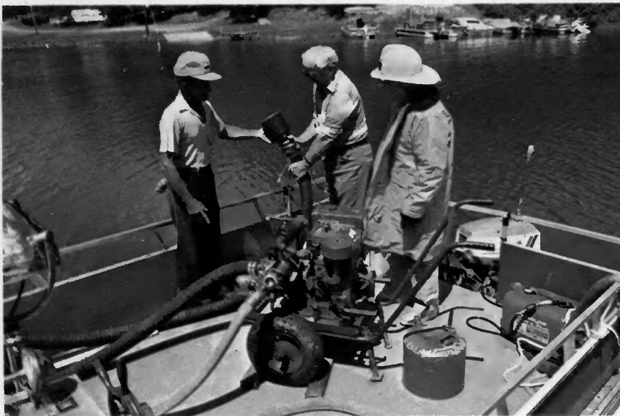
The water intake is a key element in the water delivery system of the fireboat. Duncan, left, watches as Thompson checks for obstructions, while Behling, in the yellow outfit, looks on.
