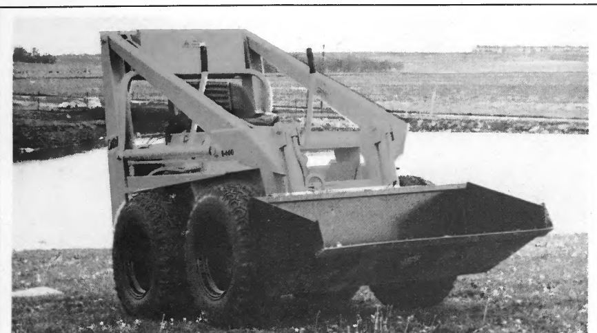
Oaks Mfg. Inc., Oaks, N.D., introduces Model L600—New—Compact—4 Wheel Drive Loader. Hydrostatic Drive—Turns in its tracks—Operation is smooth and easy...and economical to own. Ideal for any job on the farm, construction, factory and warehouse. Various buckets and forks available.
