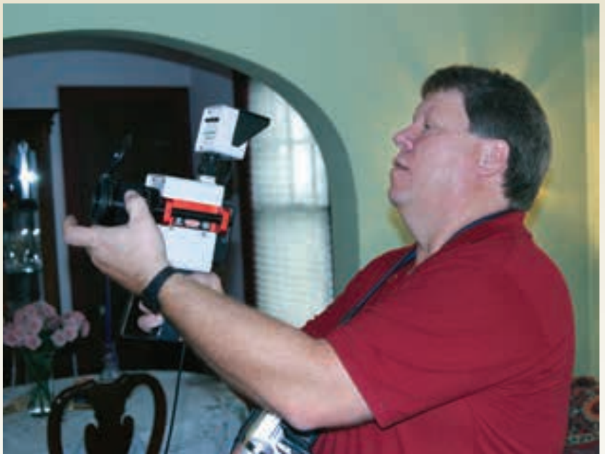
Professional home energy auditors use infrared cameras to picture energy leaks.
