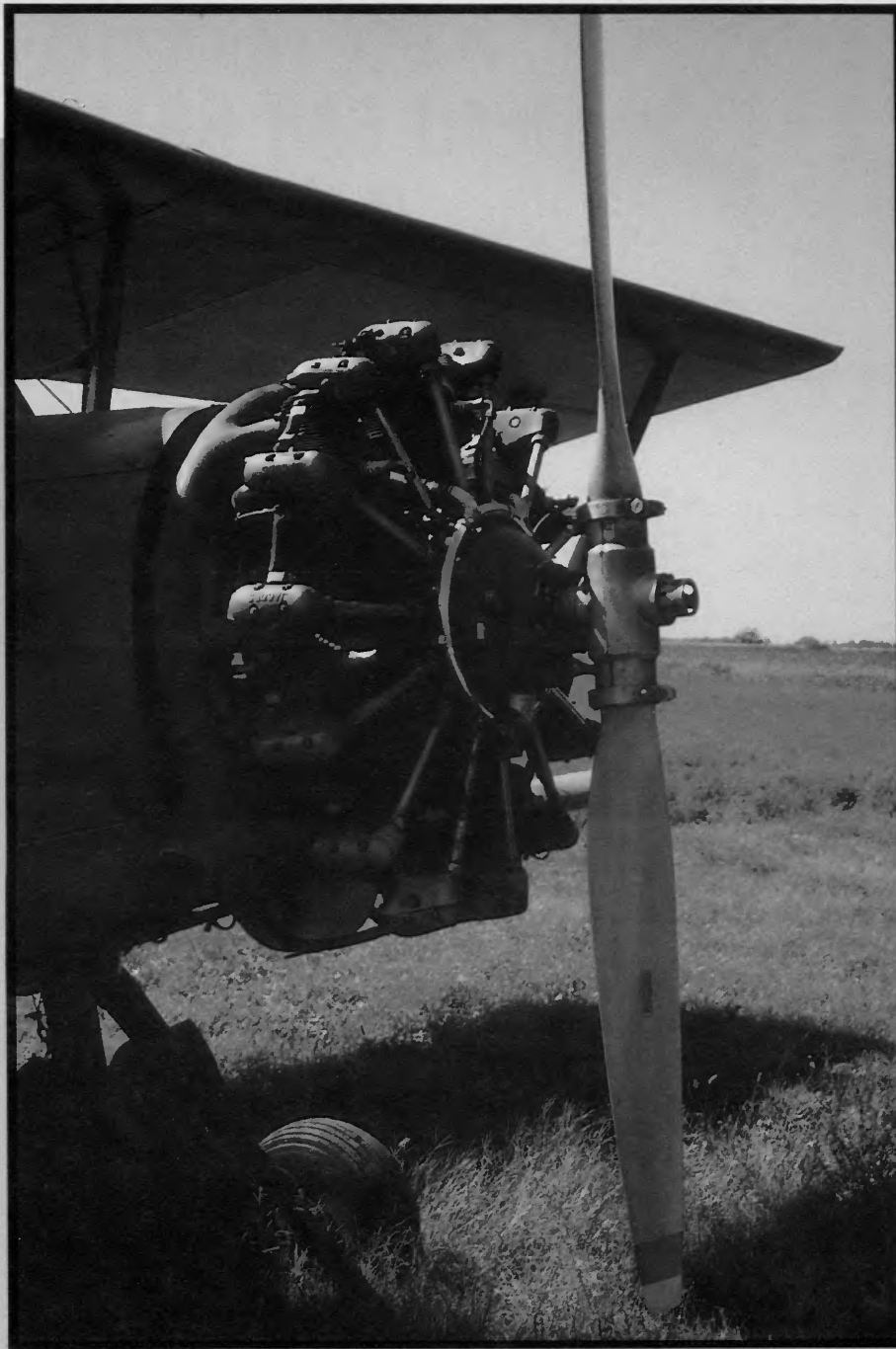
Clockwise from above: The 275-horsepower Jacobs, a seven-cylinder radial engine, powers Zumwalt's Ag Cat, getting him in and out of small fields. The Grumman Ag Cat, a sturdily built plane, carries its load in a hopper just in front of the cockpit. Joe Zumwalt in his plane.
