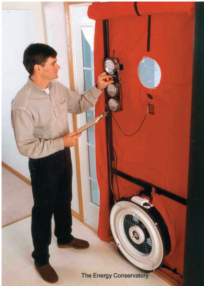
This photo depicts a blower door test, which is used to analyze a home's energy efficiency.
