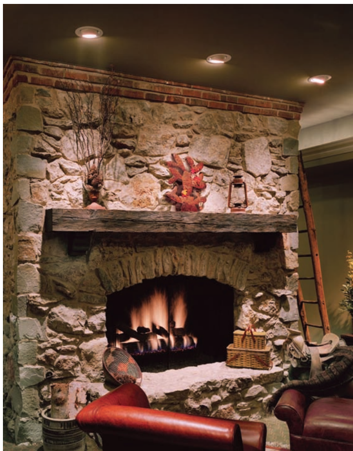
Adjustable eyeball recessed light fixtures are ideal to focus light on a specific object on the wall or floor.
