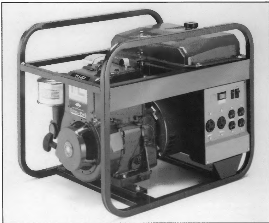
A portable generator like this one can be a big help during an outage, and can be useful around the home, too. Note the receptacles to plug appliances into. If you connect the unit into your house's wiring, you'll need a double-throw switch.
