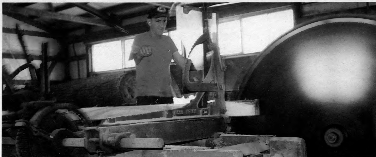
Above: Wayne Hendrix runs a log through his sawmill. With a couple of helpers, he can run some 10,000 board feet through the mill in a day.
