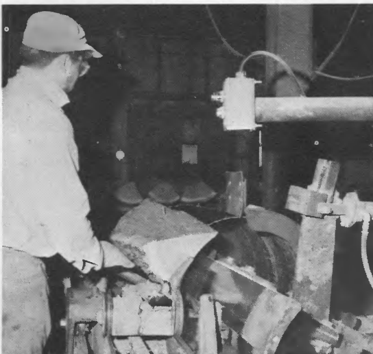
Stave bolts go through an "equalizer." Fluorescent lights above cause string to cast a shadow on the stave bolts, and accurately indicate where the bolts are to be cut.
