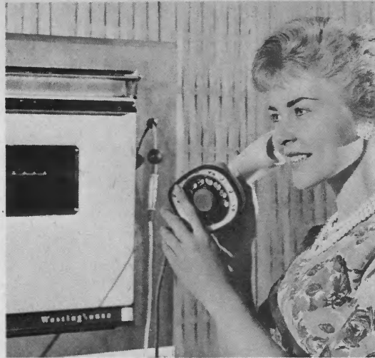
Engineers have devised a system for turning electrical appliances on by merely dialing home phone number.
