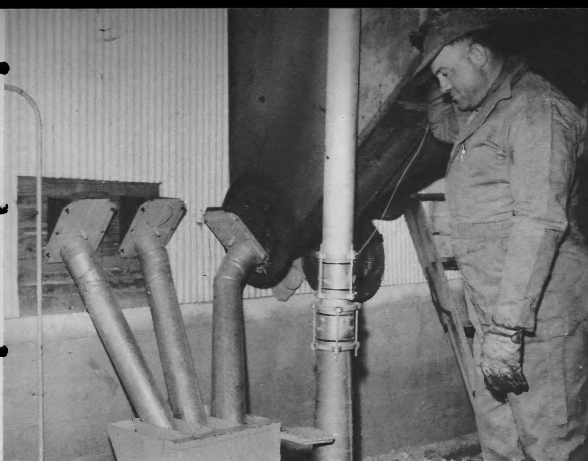
Heart of automatic, electrically-powered feed system is mix-mill in pit. Grain is channelled into it through pipes from bins.
