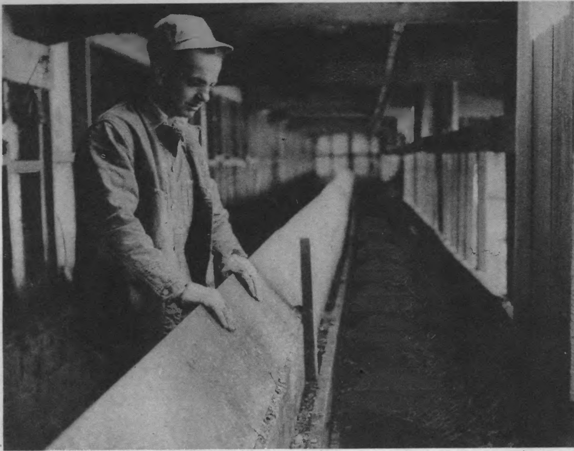
Harold Smith's bunker feeder distributes silage over 102-foot trough in eight minutes, eliminating a hard job.
