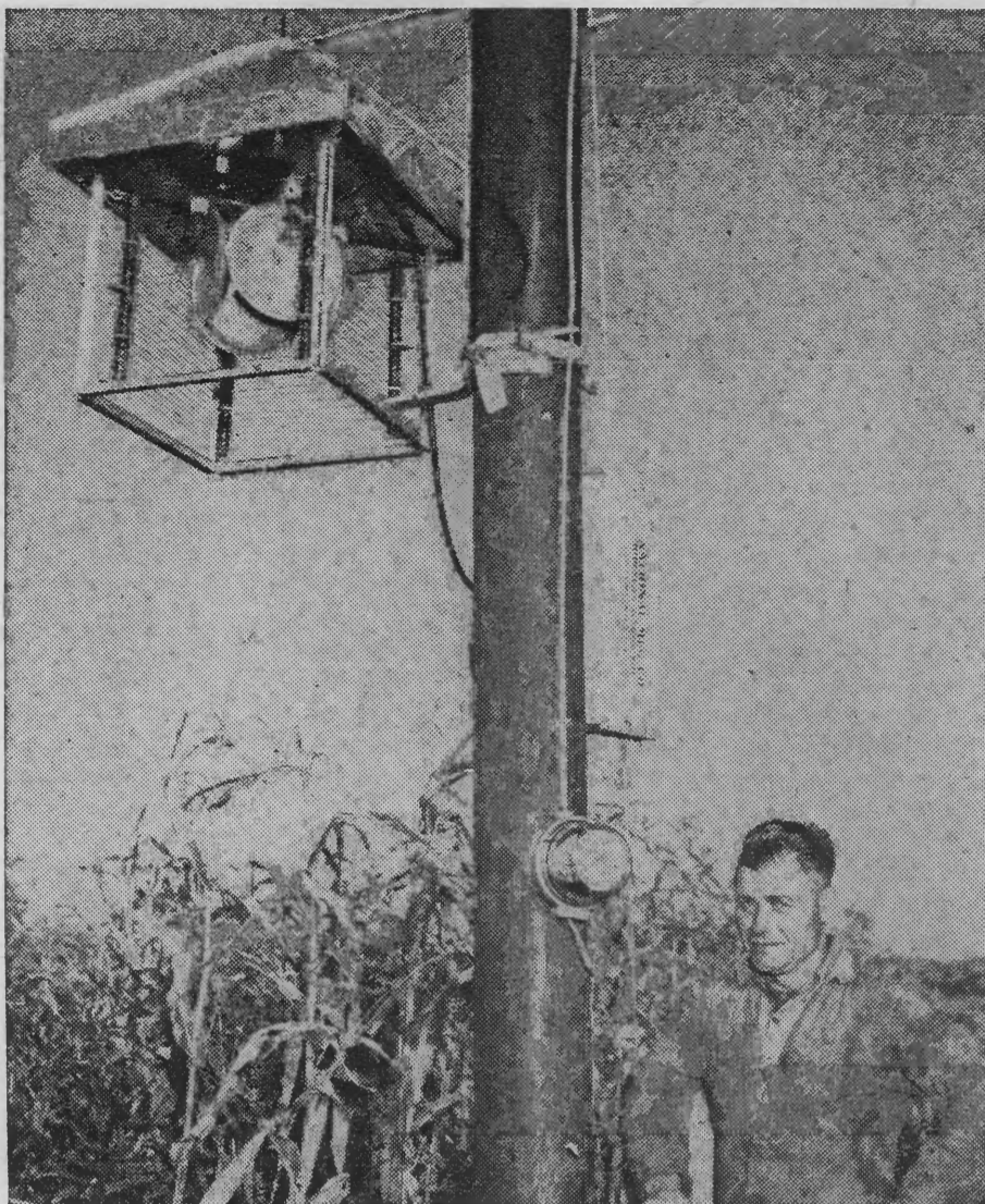
CORN BORER trap, which Boyd Handel (shown) of Chadwick tested in a 40-acre corn field last summer to determine its effectiveness. Four lights attract the moths, which are electrocuted when they come in contact with the network of wires around the trap.
