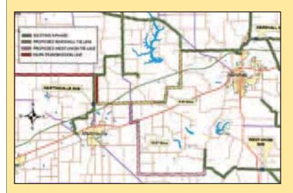
Upon completion of the substation, EnerStar anticipates constructing two tielines, represented by a pink and a yellow line. When complete, the coop will link all EnerStar substations and have the ability to "back feed" subs during an extended outage.
