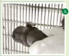
Gently vacuum and clean the coil. Using the brush or crevice attachment, carefully vacuum the dust and dirt wherever you see it. If you have pulled the fridge out, vacuum and wipe down the sides and back of the fridge and the floor.
